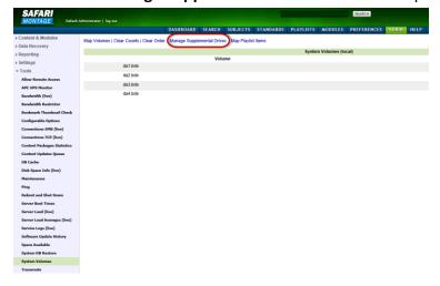
7. Link the supplemental drive to the installed content drive(s) by clicking on the **Link** action. When linking is complete, click **Return to Supplemental Drive Management** to verify the link status and link an additional drive.
